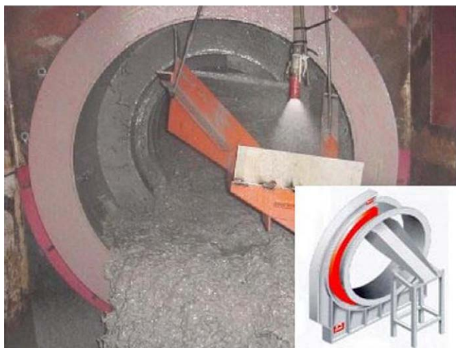
Fig. 4. A ball mill separator from Eriez. Separation of ball mill grinding ball segments from the discharge. From Eriez Magnetics, Inc.
