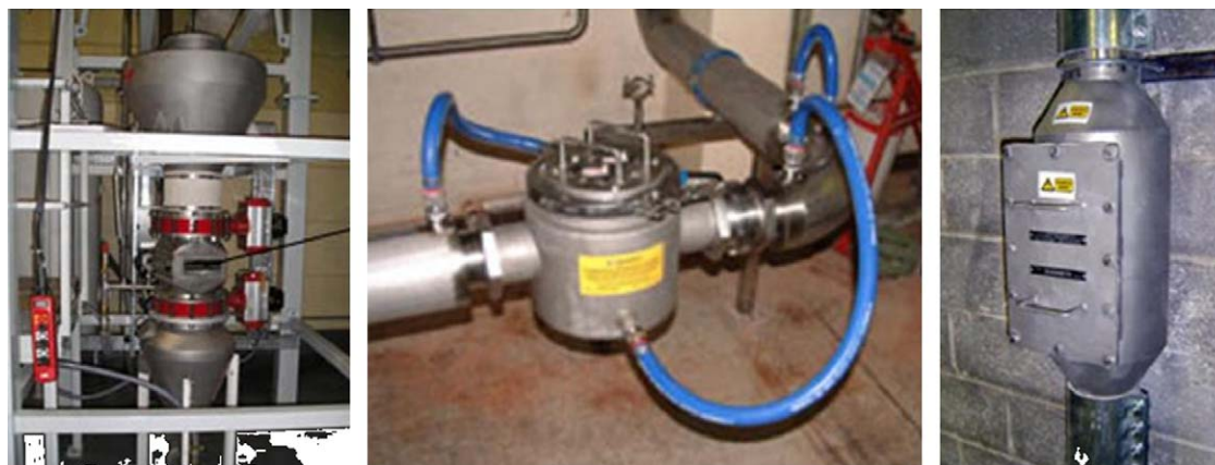
Fig. 7. (Left) A single row easy-clean grid box which contains high-density rare earth easy-clean magnetic tubes filters loose tea with a flow rate of 5 tph. (Middle) A water-jacketed pipeline magnet was manufactured to suit a 4 in pipeline pressure resistant up to 10 bar, nine high intensity rare earth magnets (11500 G) filter liquid chocolate flowing at 300l/min. The pressurized heated water-jacket maintains the temperature of the chocolate. (Right) The Bullet magnet that is used by a flour producer in which flour flows upwards through the 5 in pipe and any ferrous contamination is removed by the high intensity rare earth bullet magnet (8500 G min).
